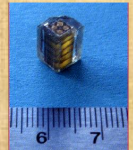
Transducer stack for ultrasonic sonar application (TRS Ceramics)
